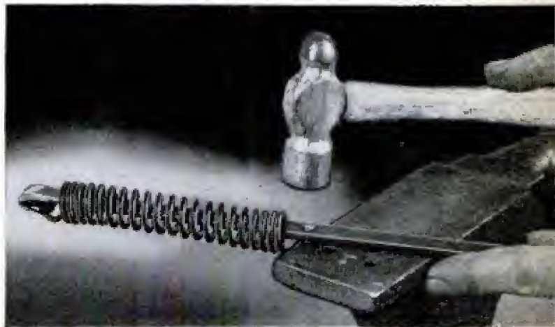
Toaster handle is fitted with "cool" grip formed by riveting coil spring to looped end of flat steel rod
